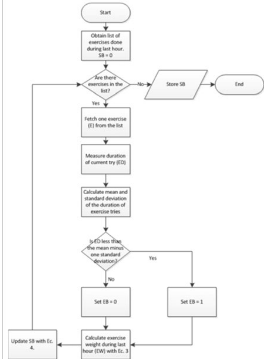
Figure 4: Flow of rules for the detection of boredom
